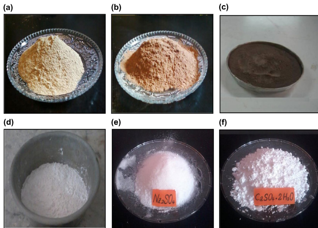
1 Materials used a grey soil sample b red soil sample c natural pozzolana powder d hydrated lime e Na_2SO_4 and f CaSO_4 \cdot 2H_2O
